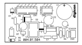
The anti-panic system requires a power of 12Vcc 2A. Optionally, Digicon also provides a switched-mode power supply (code 019.01.334). To avoid overheating of the solenoid, the control board has an automatic routine that reduces its voltage to 6Vcc two seconds after the turnstile is tuned on. One disassembled, the arm should be placed manually back into position.
